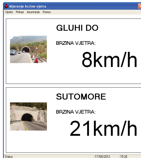
Fig. 7. The numeric display shows current wind speed at tunnel portals.
